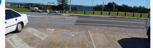
There are more than 50 car parking bays in the area. Two are marked mobility parking bays. The mobility parking area is concrete, 2.6m wide and 6m deep, with a shared 2m gap between the parks.
